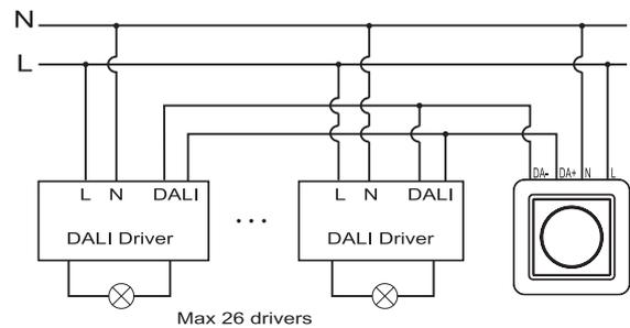
Set Dip switch to broadcast. All devices, max 26, would be controlled as a group.
